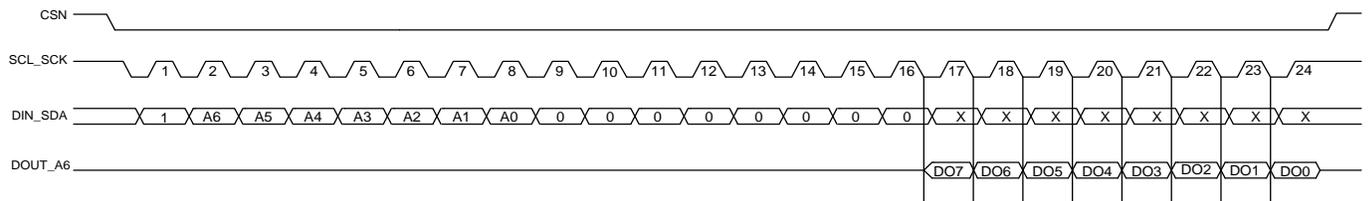
**Figure 17. SPI Register Read Cycle - Single**
