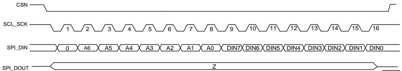
Figure 15. SPI Register Write Cycle - Single
